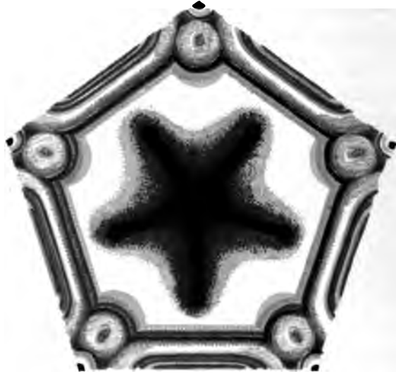
CHROMATIC EFFECTS OF A PENTAGON OF UNANNEALED GLASS IN POLARIZED LIGHT.
